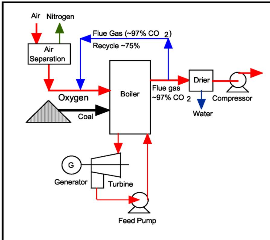
Figure 2 Oxyfuel combustion
