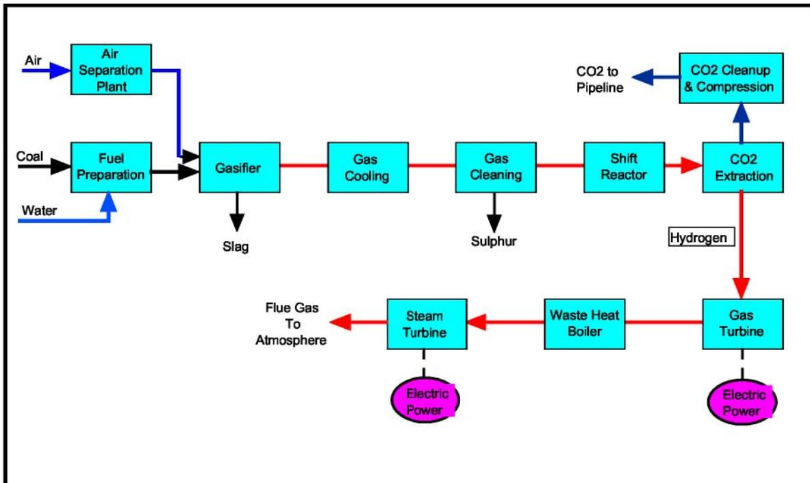
**Figure 3 Coal gasification**
