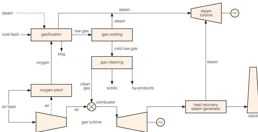
*Integrated gasification combined cycle without CO<sub>2</sub> capture – major component systems*
