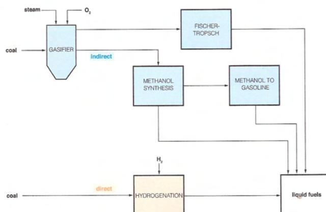
**Figure 5 Principal process routes for the production of liquid fuels from coal (Couch 2008)**
