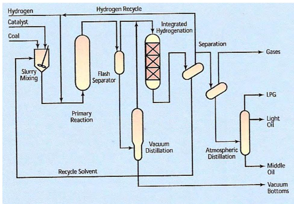
Figure 8 The DT Process (DTI 1999)
