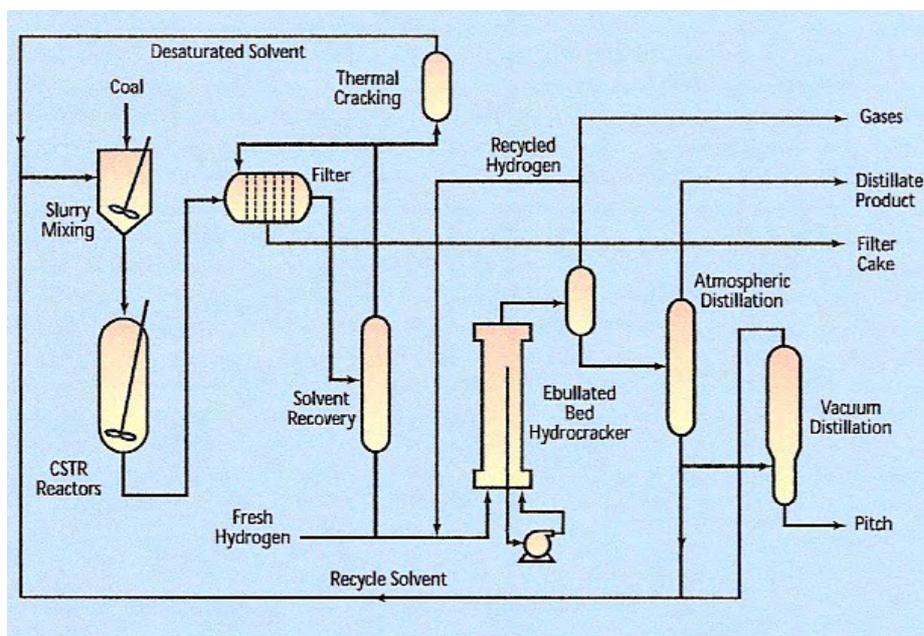
Figure 9 Schematic of the LSE process (DTI 1999)
