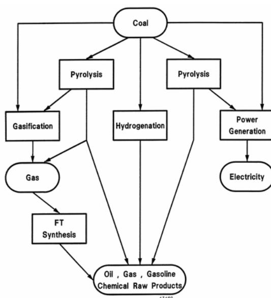
**Figure 7 Hydropyrolysis as an approach for coal-to-liquids conversion (van Heek and Wanzl 1989)**
