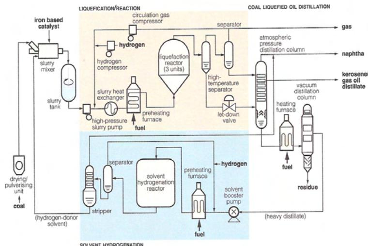
**Figure 13 NEDOL process flowsheet for bituminous coal (NEDO, 2006)**
