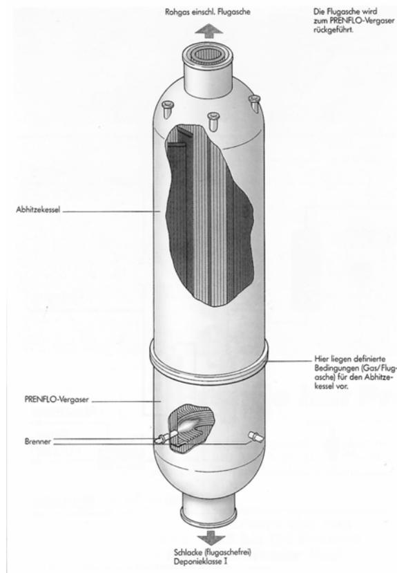
**Figure A4 Prenflo Gasifier with radiation boiler**
