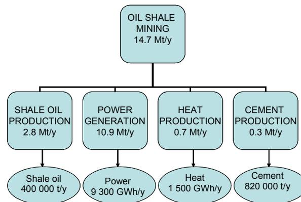
**Figure 4 Material flows in the Estonian oil shale industry (Länelaid 2009)**
