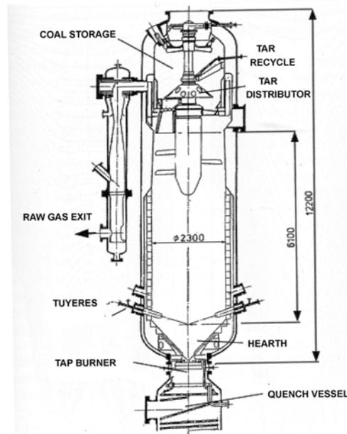
**Figure A2 BGL Slagging Gasifier**
