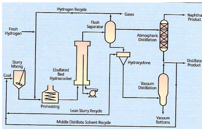
**Figure 17 Schematic diagram of the H-Coal process (DTI 1999)**
