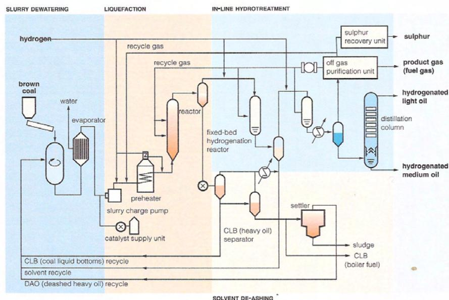
**Figure 14 NEDO brown coal liquefaction process flowsheet (NEDO 2006)**
