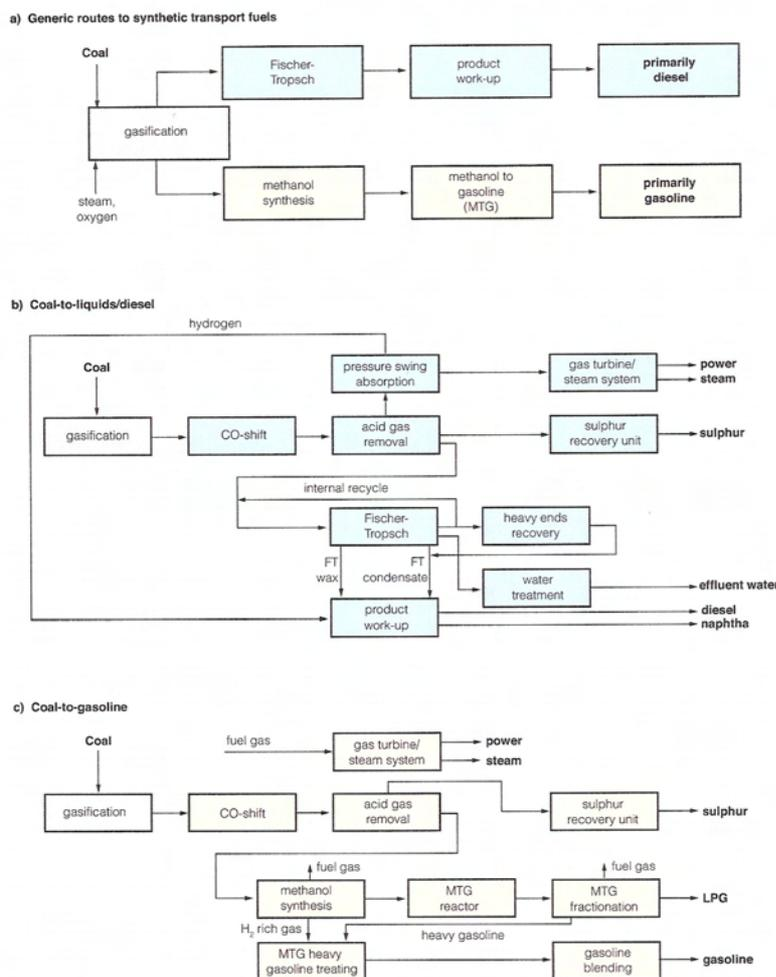
**Figure 6** Flow diagram of the two generic routes to synthetic transport fuels using ICL (Radtke et al 2006)
