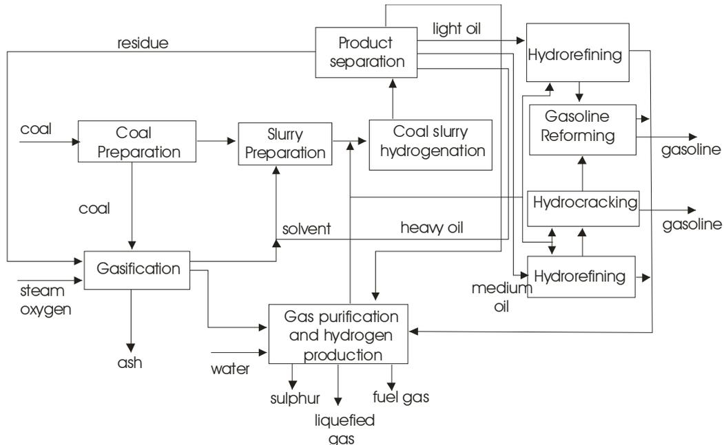
**Figure 11 CTL process based on the Central Mining Institute concept (CMI 2006)**
