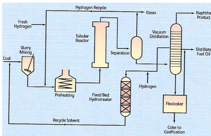
**Figure 18 Schematic diagram of the EDS process (DTI 1999)**
