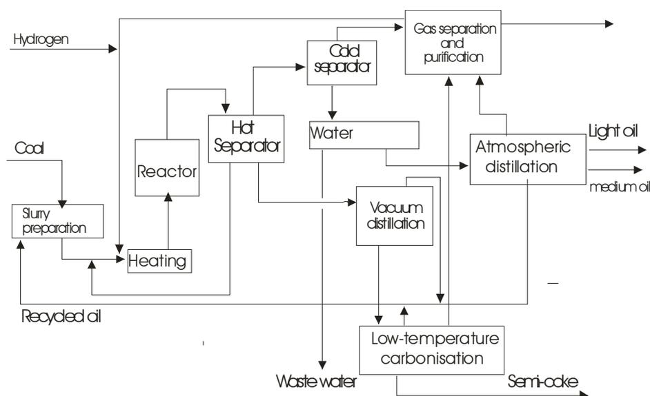
**Figure 10 Central Mining Institute direct coal hydrogenation process**
