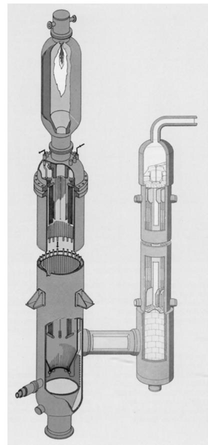
**Figure A5 GE Energy wet feed entrained coal gasification**
