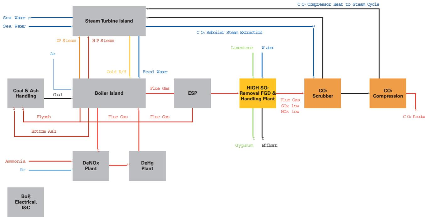
Figure 11 below presents an indicative diagram for an Oxyfuel CO<sub>2</sub> capture system. For low sulphur coals the flue gas desulphurisation (FGD) plant can be omitted. An air separation unit is used to separate the oxygen and nitrogen, and the coal is burnt in oxygen diluted by recycled flue gas (predominantly carbon dioxide). This has the advantage of significantly concentrating the CO<sub>2</sub> concentration.
