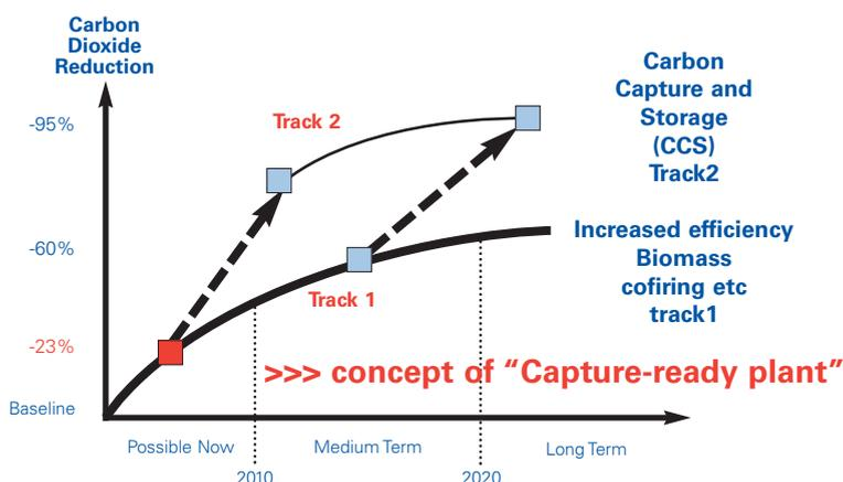
The Track 1 approaches are available now. They bring reduced CO<sub>2</sub> emissions per unit of electricity generated. Track 1 approaches include improved efficiency by introduction of Advanced Supercritical (ASC) boiler/turbine technology and biomass cofiring (substitution of up to 20% of the coal fuel by biomass which is CO<sub>2</sub> neutral). More detail is given in section 3.2 on Mitsui Babcock's preferred technology and in section 3.3 on alternatives.
