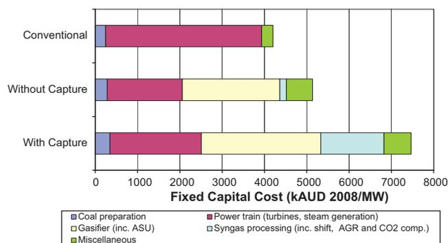
**Fig. 4 – Fully installed capital costs for the three power plants in Australian Dollars per MW of installed capacity showing the breakdown between the four main sections of the process for a coal consumption rate of 4369 tonne d<sup>-1</sup>. The miscellaneous section refers to water treatment, the cooling water system and the outside battery limits of 5% of the inside battery limits capital.**
