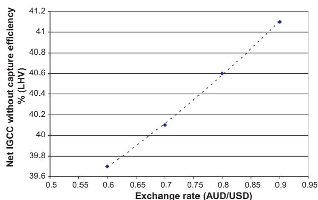
**Fig. 8 – The required efficiency for IGCC without capture to match the selling price for conventional coal electricity as a function of the AUD/USD exchange rate.**
