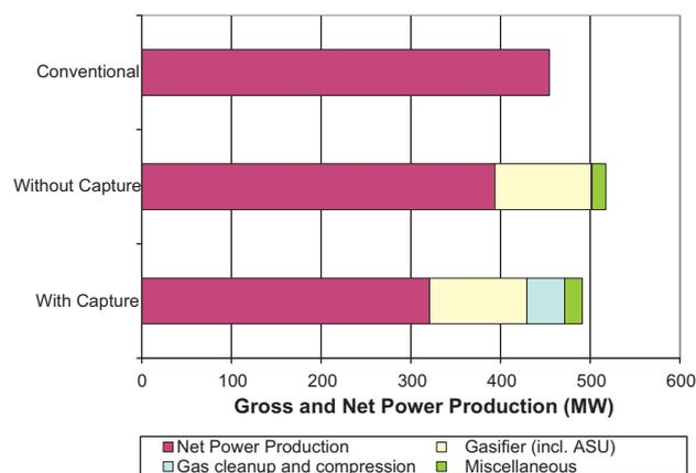
**Fig. 3 – Gross and net power production showing the consumption within the different sections of the IGCC process for a coal consumption rate of 4369 tonne d<sup>-1</sup>.**
