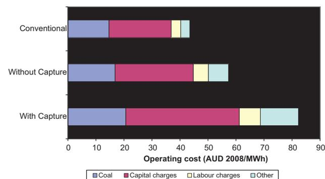
**Fig. 5 – Specific operation costs in Australian Dollars per MWh of net electricity production for a coal consumption rate of 4369 tonne d<sup>-1</sup>.**
