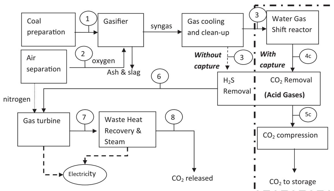
Fig. 1 – Block diagram for the IGCC process with/without CO<sub>2</sub> capture.
