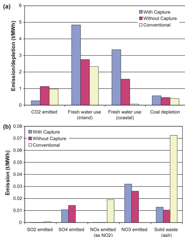
**Fig. 6 – Inventory data per unit MWh of net electricity production: (a) higher mass inventories and (b) lower mass inventories.**
