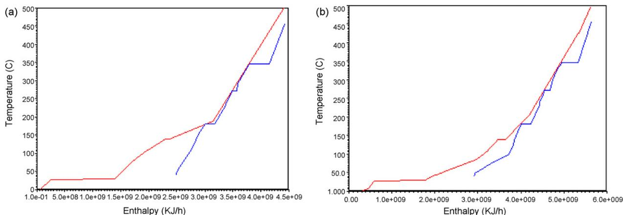
Fig. 2 – Shifted composite curves for IGCC (a) Case B and (b) Case C.
