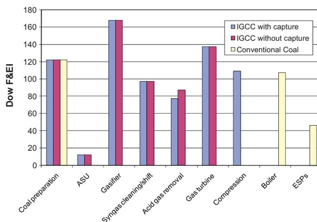
**Fig. 7 – The Dow fire and explosion index for the different zones within each process.**
